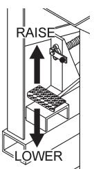
Figure 26. Raise/Lower Step Pedal
